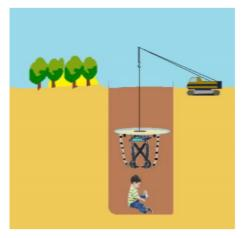
Fig 2 Robot used for rescuing child inside the borewell
