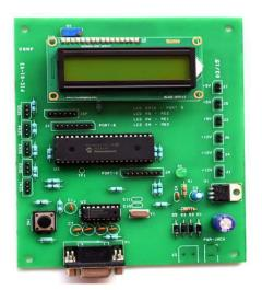
FIG 6: PIC ASSEMBLED PCB+UART+LCD
